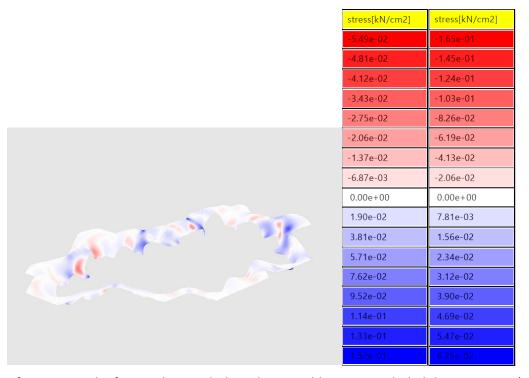
After running the first analysis with the values in table 2 we concluded that our young's modulus was incredibly low. According to literature the maximum allowable tensile stress for earth constructions is between 10%( Martins, T.,2006) and 20%(NZ 4297,1998) of the compressive strenght. Meaning that the maximum tensile stress should be below one fifth of the compressive strength.
